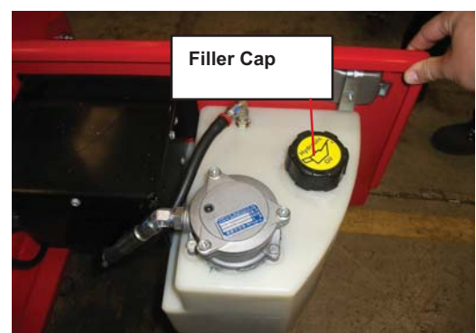
Figure 8: Hydraulic Fluid Reservoir and Dipstick
